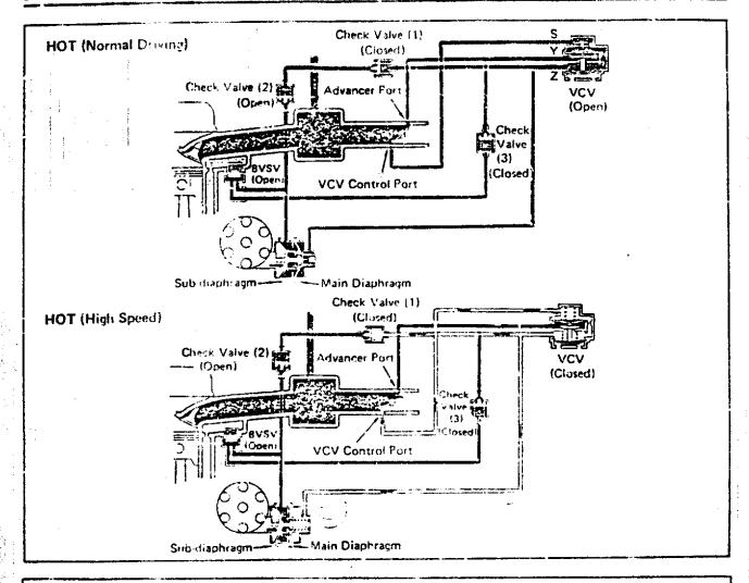
To improve cold engine performance, this ignition system advances the ignition timing when the engine is cold, and to improve idle performance, advances the ignition timing when there is a load on the engine. The distributor is equipped with two diaphragms that have different vacuum advance characteristics.
